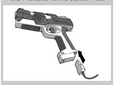
Push the sensor vest connector upward in its housing until you hear a clic.
