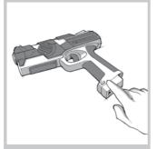
Remove the battery pack by pressing the battery pack button and pulling the battery pack downward.
