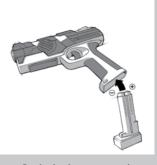
Push the battery pack back in its housing
